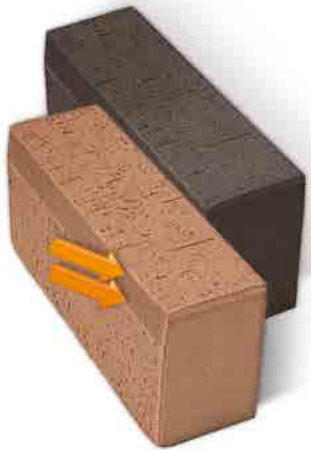
Tapered spacers combined with a mini chamfer protect the clay pavers from spalling.
